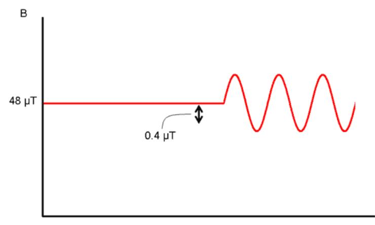
The AC field is often less than the DC field. In fact it's often very much less. This example, not drawn to scale, shows the 0.4  $\mu$ T AC field implicated in the epidemiology of childhood leukaemia with the typical 48  $\mu$ T geomagnetic field in the UK. (0.4  $\mu$ T is the rms value, the peak is slightly higher, see a tutorial on ways of characterising AC fields.)
